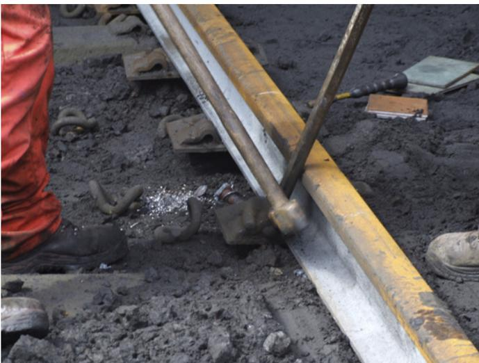
Coated rail being levered and hammered into position using a 7kg sledge hammer. A perfect response to questions asked about the impact-resistance of the Zinga coating!
