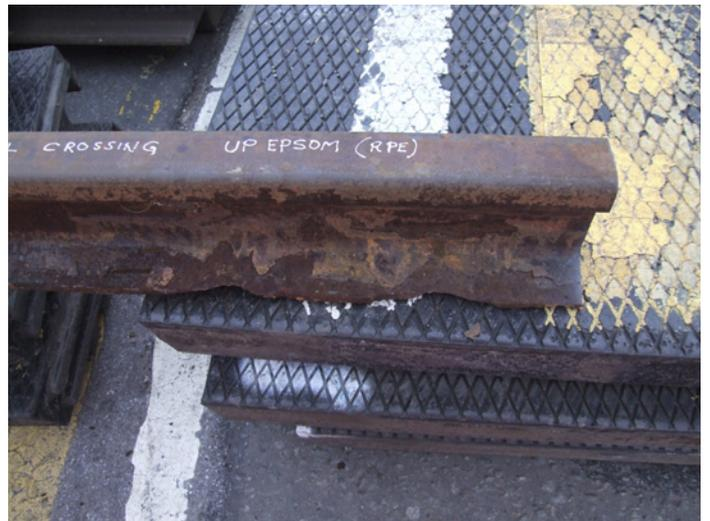
A corroded rail from the West Barnes crossing in East London clearly demonstrates that a rail with a predicted life of six years was written off within three months. It was this incident that triggered the whole rail-coating process and was followed by six years of intensive research and trials.
